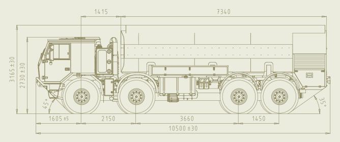
The TATRA 8x8 fuel tanker is suitable for operation in the most difficult off-road or cross-country conditions. The vehicle can be used for transporting of fuel to different reservoirs or for direct filling of smaller refuelling tankers. Design and equipment according international standard for transporting of danger liquid - ADR - code LGBF and other STANAG standards.
