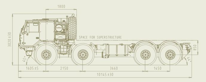
cal truck, or carry various kinds of special superstructures and load handling systems. Exceptional resistance of the chassis against twist and bending, as well as low transfer of vibrations on the load make it ideal means for transporting standard containers and shelters, sophisticated electronics, or other sensitive loads.
