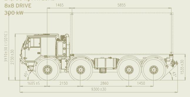
cal truck, or carry various kinds of special superstructures and load handling systems. Exceptional resistance of the chassis against twist and bending, as well as low transfer of vibrations on the load make it ideal means for transporting standard containers and shelters, sophisticated electronics, or other sensitive loads.
