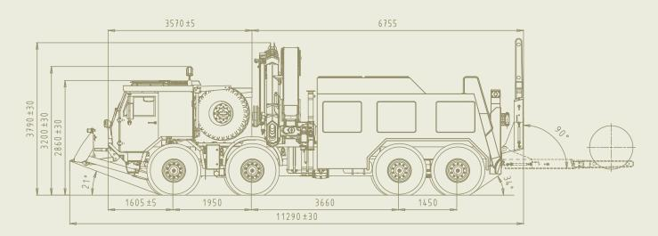
The High Mobility Heavy Duty (HMHD) Recovery Vehicle is able to recover armoured vehicles very quickly and efficiently in a tactical environment. The vehicle capability and payload enabling to recover heavy armoured vehicles and it is capable of towing most types of current and future wheeled vehicle systems and their variants. The vehicle is
