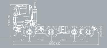
Other possible standard wheelbase: axle 2-3: 2,560/2,950/3,360 mm axle 3-4: 1.450 mm
